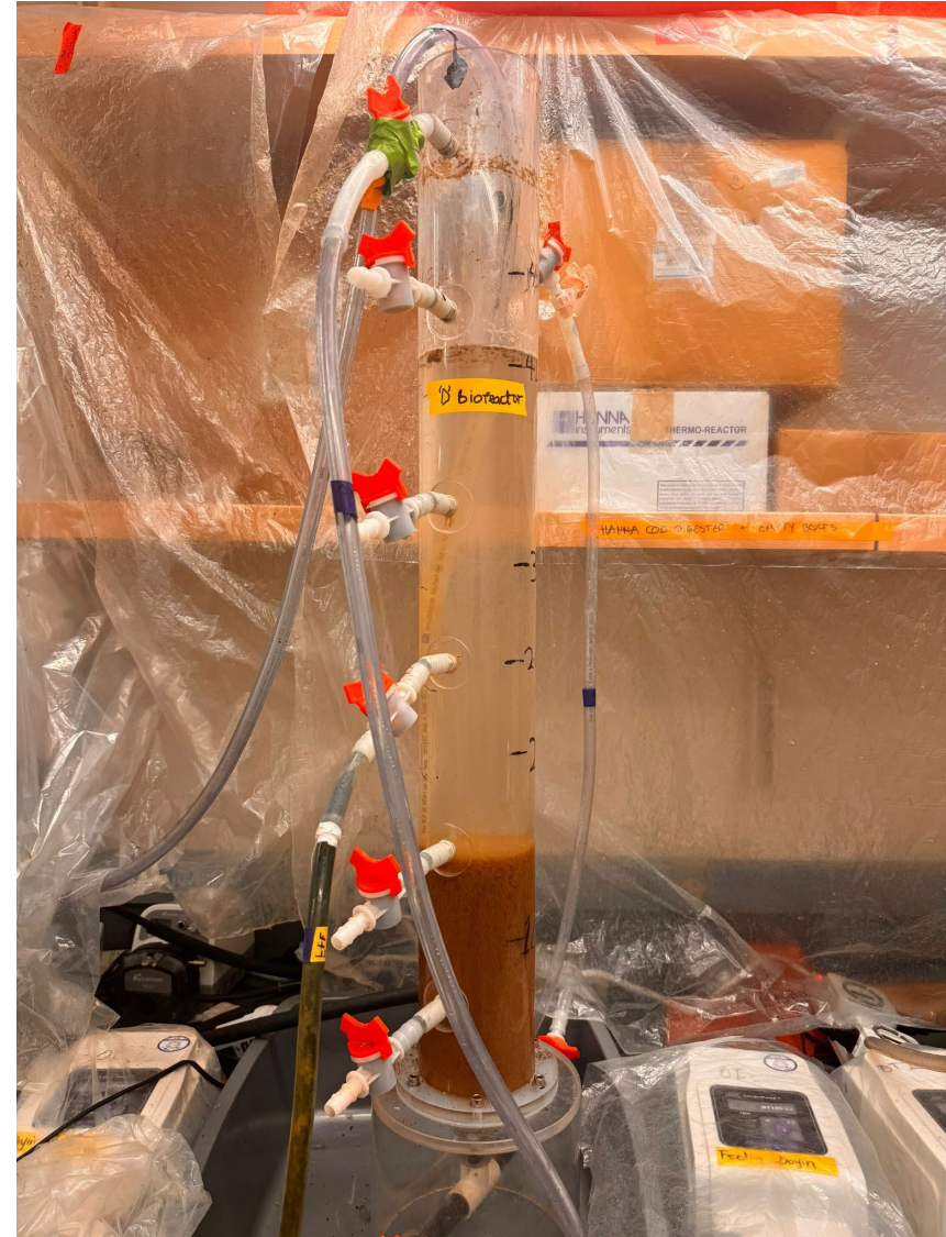
Fig 5b: Bioreactor during settling phase
