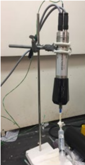
Sensor calibration with sulfide standard
