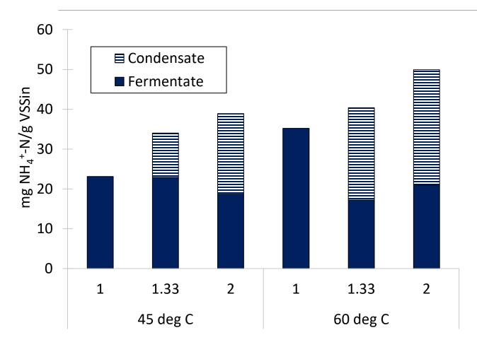
Fermentation Impact: reduced ammonia in the digestate. Condensate is very clean water, suitable for resource recovery
