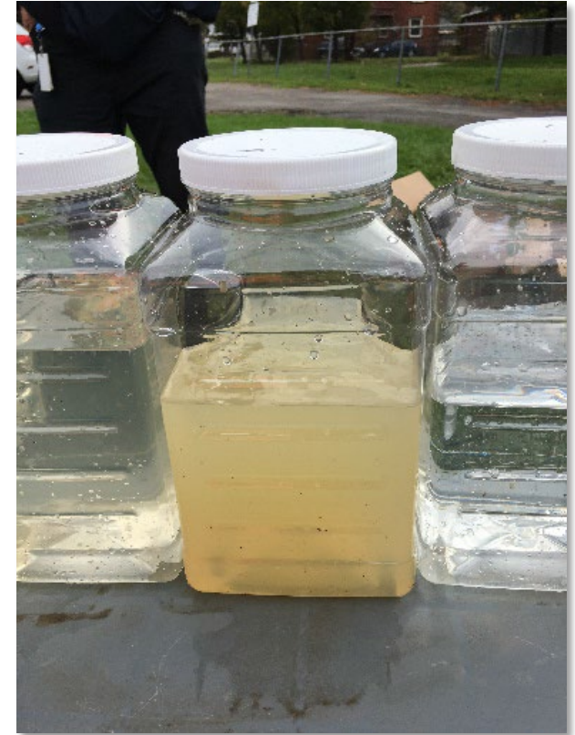
Flush water containing 38 mg/L aluminum
